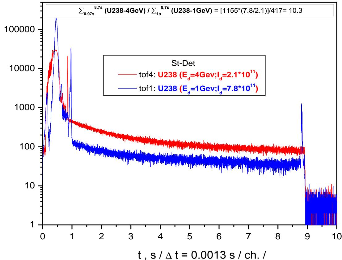
**Time dependent neutron spectra from St-detector for natural uranium target irradiated by deuterons with energy 1 and 4 GeV.**
