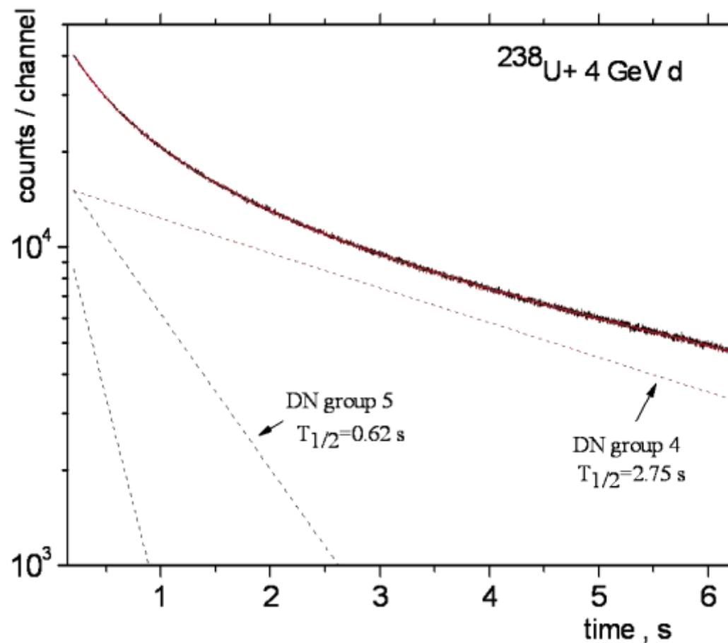
Decomposition of DN spectrum for  $\text{U} + \text{d}$ ,  $E_d = 4$  GeV
