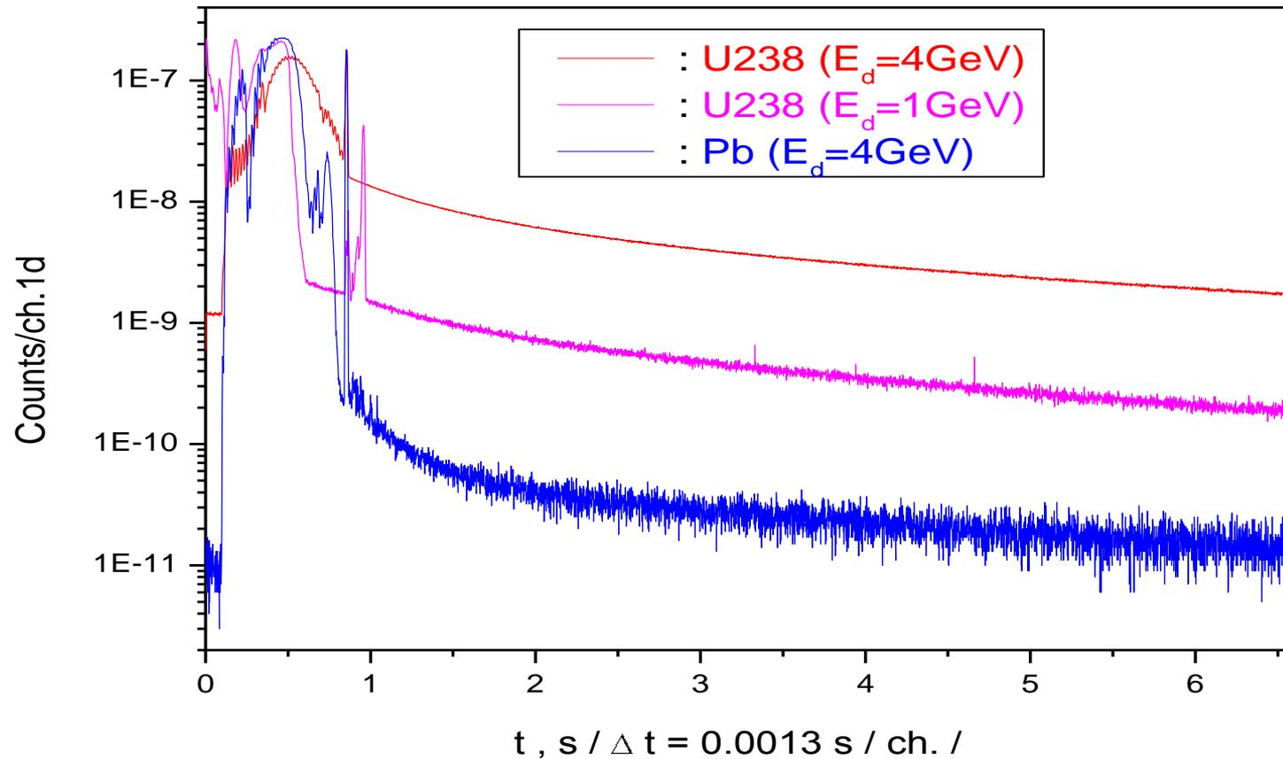
Time dependence of neutron yields from a geometrically identical target assemblies of lead and lead-uranium irradiated by deuterons with energy of  $E_d = 1$  and  $4$  GeV
